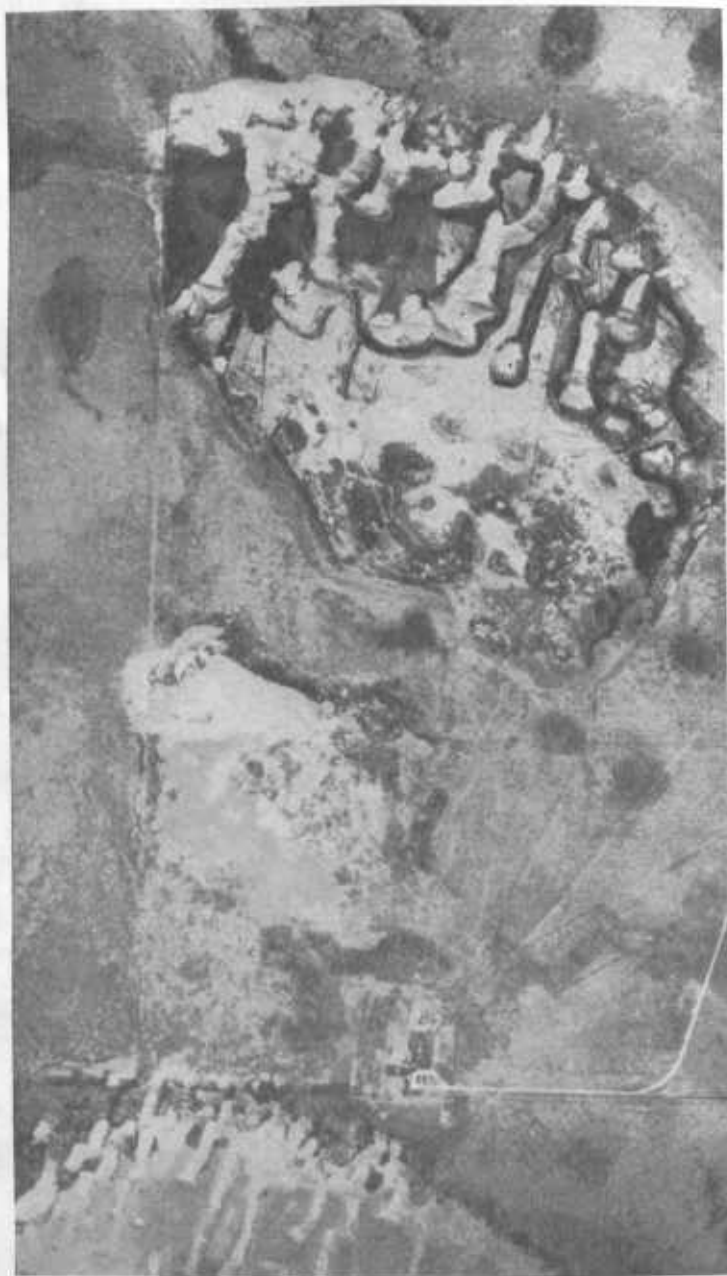
FIGURE 4.—Aerial photograph of the sand-dune study area. On the extreme left is the untreated check area, with dunes and hard eroded land. On the right is the dune site that has been treated. Listing around the dunes and wind channels across the dunes are shown.
